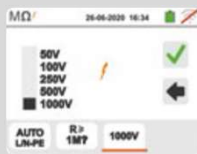
SELECTION OF TEST VOLTAGE AND MINIMUM LIMIT VALUE ON MQ MEASUREMENT
