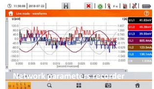
power quality analyzer
