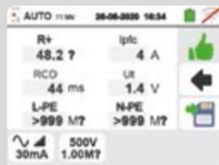
AUTOSEQUENCE: MEASUREMENTS OF RESISTANCE OF OVERALL EARTH RESISTANCE, RCD TEST AND INSULATION L-PE, N-PE
